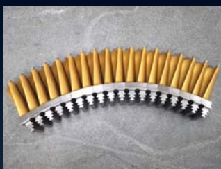
Side-entry blades with Titanium nitride coating
